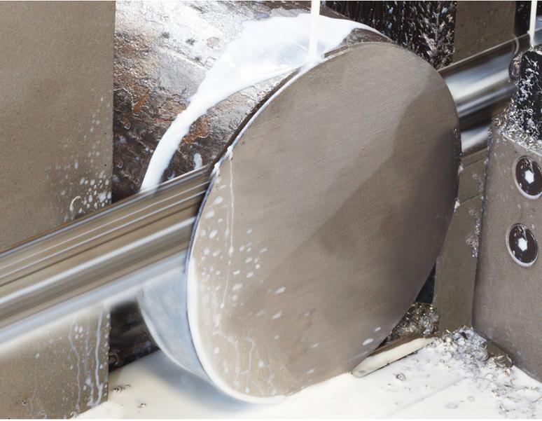
Sawing is one of the oldest cutting techniques in use today, and innovations have allowed the process to keep up with advances in material, tolerances and product complexity. By definition, sawing is cutting a narrow slit in a workpiece by moving a toothed or abrasive cutting tool against the surface. Sawing is often used to remove large sections of material without particular concern for tolerances, but modern CNC sawing machines can be used for finishing work as well.
