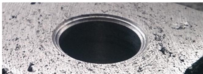
Above: a stepped hole formed by drilling
