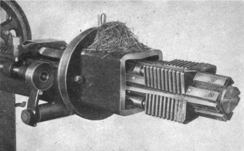
Broaching is a machining process using a cutting tool with teeth that increase in size from front to back. In many cases, an entire surface (or multiple surfaces) can be finished in a single pass with broaching. The technique is most often employed to finish holes, splines and flat surfaces.
