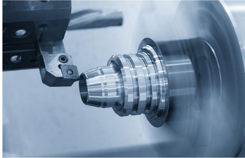
*Above and opposite: turning processes on a CNC lathe*
