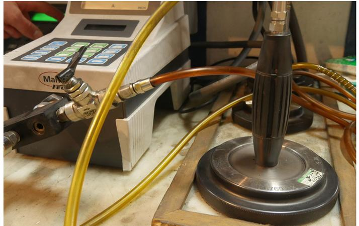
Air gages use pressurized air to measure the dimensions of an object. They were first introduced in the 1940s, and have undergone improvements to become one of the most trusted precision measuring tools in machine shops. Air gages function by shooting air out of a specifically calibrated nozzle, and recording the rate at which the air returns to multiple sensing nozzles. Thus, they are able to read the air flow between the measuring tool and the object being measured.
