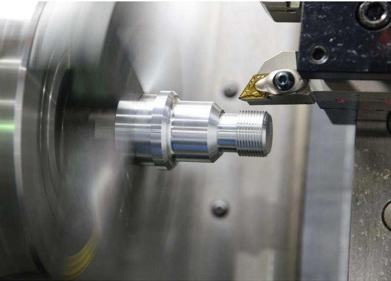
Turning has been practiced by machinists for centuries on many different materials. Originally, turning acted on wood to create complex, cylindrical designs for use in tools, handles and furniture. Today, turning is a vital part of the metal manufacturing process, and a major technique used by precision CNC machine shops around the world.
