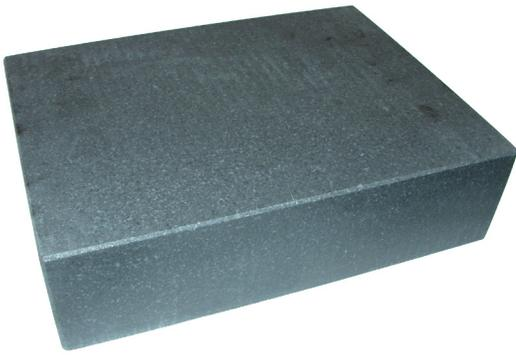
A surface plate is a flat surface used as a reference point for vertical (Y-axis) measurements. They're only useful if they're properly calibrated and maintain their shape impeccably. Because of its smooth surface and low level of expansion and contraction with temperature changes, granite is often the material of choice for surface plates.
