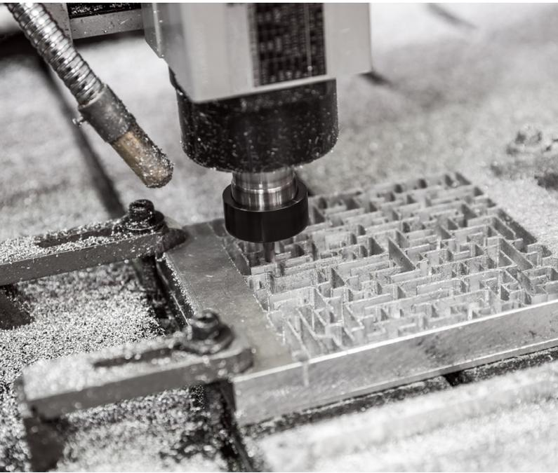
**Milling** is one of the most common processes in CNC machining, most likely because it is so versatile. Using a single tool, machine shops can create contours, shapes and angles on the surface of a workpiece. Milling can completely transform a piece of metal stock into a finished part of nearly any complexity.
