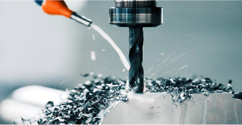
**Drilling** is one of the most common techniques used in manufacturing to create holes. In contrast to other hole-making methods like boring, reaming and tapping, drilling is most often used to create holes in unbroken surfaces. In precision CNC machining, drilling can range in scope from simple, rough hole drilling to complex, multi-feature hole drilling.
