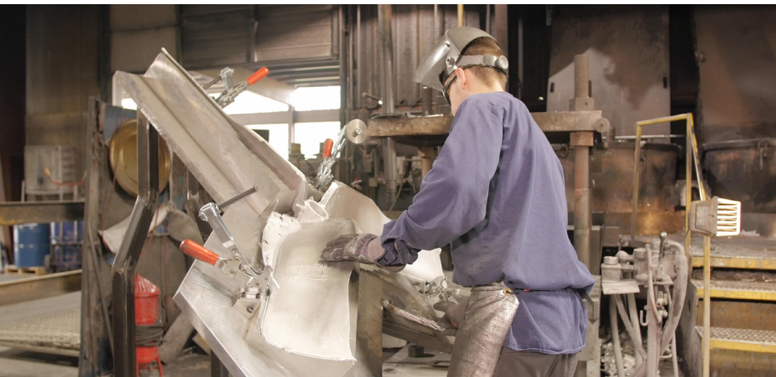
Left: Eagle Aluminum operator mounts prop in cooling fixture
